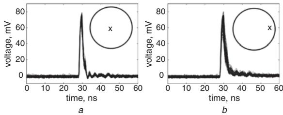
**Fig. 3** Measured received pulse laser signals with different illuminated positions in STUD
