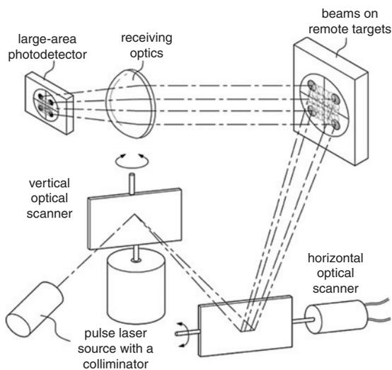
Fig. 1 3D laser radar (LADAR) with large-area photodetector
