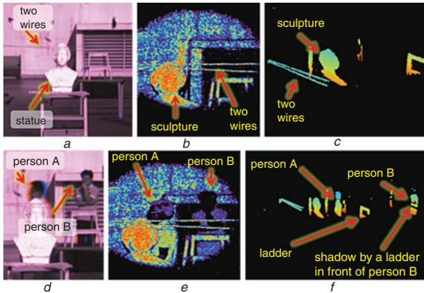
**Fig. 4** Obtained images from implemented prototype using STUD laser radar: CCD images; intensity images; 3D images
