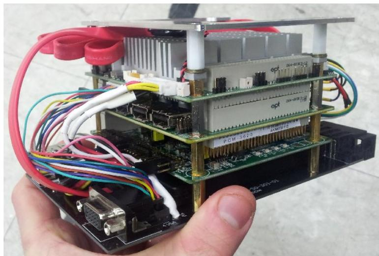
Figure 5.1: Embedded PC removed from robot, for testing the control software
